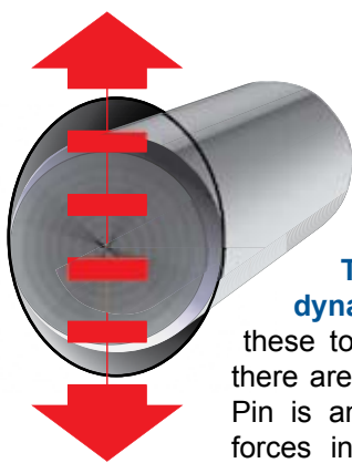
The Solid Pin's rigidity elongates the hole.
